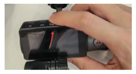
4. When the light indicator on the camera blinks, you can take your finger away from the button, and the camera starts to upgrade. It will take about 2 minutes till the camera upgraded successfully.
