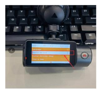
2. All the firmware files must save at root directory of the SD card.
